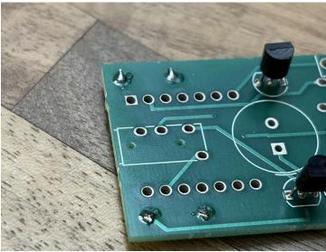
Then you can solder one of the narrow 3.5mm PCB jacks on. Put it on the white square location centered at the end of one side, as pictured below.
