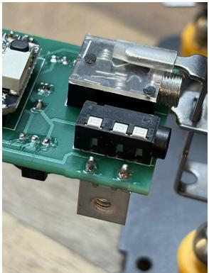
Before you put the Vail Adapter in the 3D printed case, make sure it works by powering it on. If it doesn't already have firmware flashed to it, go to <a href="https://update.vailadapter.com/">https://update.vailadapter.com/</a> and download the right firmware and install it to the arduino following the instructions on that site.
